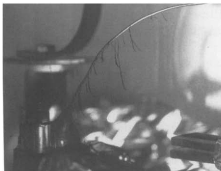
Fig. 2. Photomicrograph of vanadium fiber bundles up to 3 cm long in the apparatus. The wire voltage is on, so the fibers stand out from the wire against gravity.
