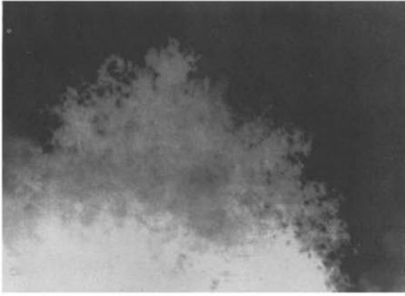
Fig. 6. Scanning electron micrograph of germanium fibers (magnification, 8100 \times ). Individual fibers are barely resolved.
