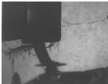
Fig. 4. Photomicrograph of silicon fiber bundles up to 0.3 cm long in the apparatus.
